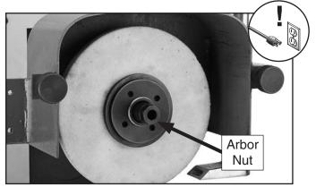
Figure 36. Wheel assembly and arbor nut installed.
